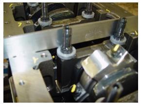
This kit includes 1 girdle, 14 top spacers, (large hole) 12 bottom spacers (small hole) 1 rear main spacer bar, 2 rear main stud nuts (12 point), and 12 main stud Ny-lock nuts.
