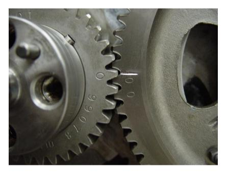
With normal engine rotation the crankshaft turns CW and the camshaft CCW. With 36 teeth on the crankshaft gear, turning the cam gear one tooth CCW will advance the cam & pump timing 10 crankshaft degrees and 5 camshaft & injection pump degrees.
