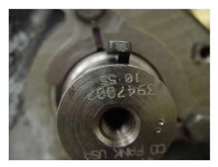
Installing the cam key as pictured with the modified cam gear will bring the cam back to a 90° intake centerline.
