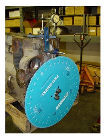
The stock cam on this 5.9 cummins is installed @ 90° intake center line.
