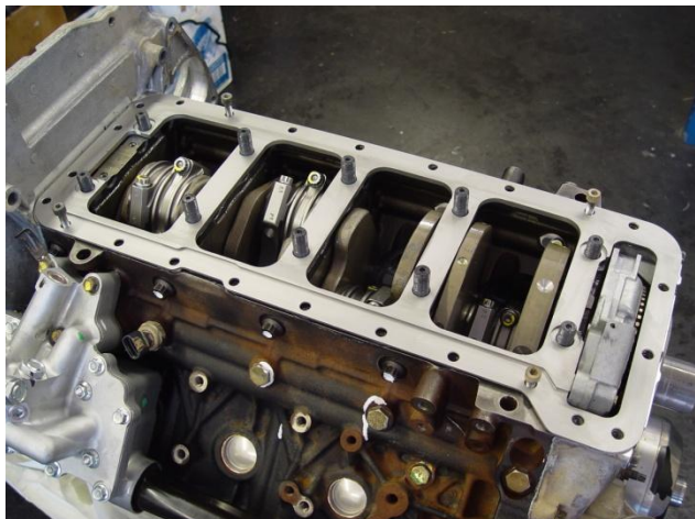
(3) APPLY A 1/16 INCH BEAD OF SILICONE (PERMATEX THE RIGHT STUFF) AND INSTALL GIRDLE.
