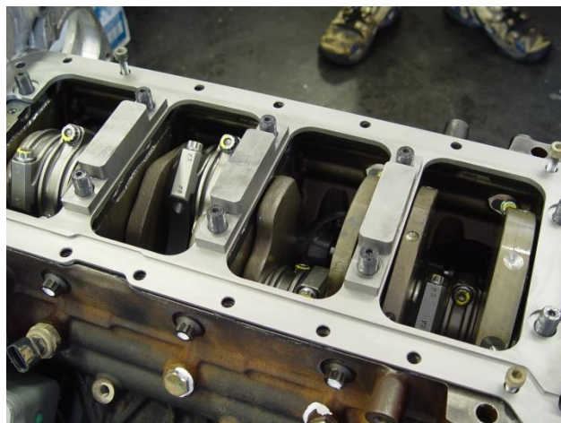
(4) INSTALL 4 OIL PAN BOLTS TO ALIGN THE GIRDLE. INSTALL 3 CENTER MAIN CAP REINFORCEMENT BARS.
