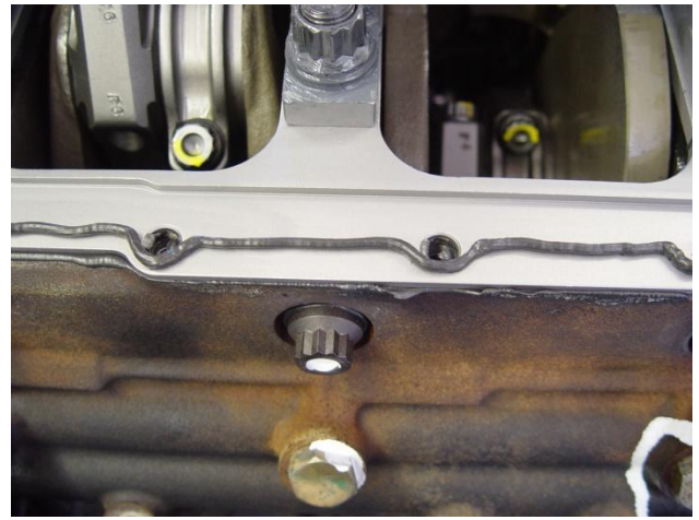
(8) APPLY A 1/16 INCH BEAD OF SILICONE TO THE PAN RAIL. (PERMATEX THE RIGHT STUFF)
